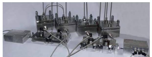
SCHEMATICS OF THE WaSul™-Perm SYSTEM FOR PERMEABILITY MEASUREMENTS AT PRESSURE UP TO 1000 BAR AND TEMPERATURE UP TO 120 °C
